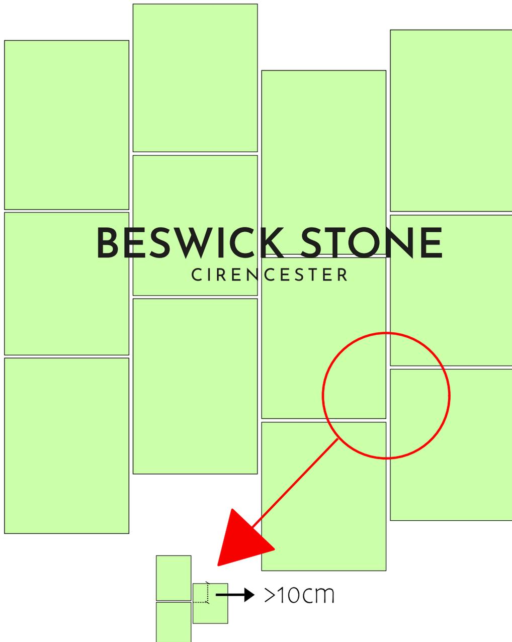
**Laying tip: there is NO pattern to follow, simply lay the tiles in straight rows, aim for no less than 10cm between the short side grout joint from row to row.**
